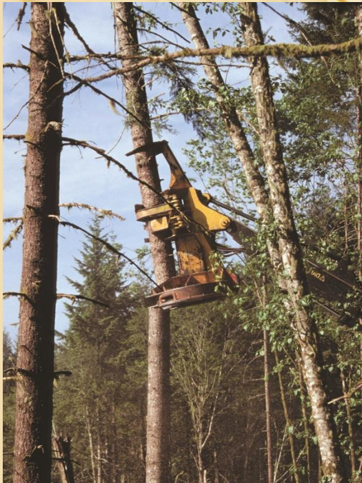
Timber-harvesting machinery, such as this feller-buncher, can be used to create snags by topping live trees. Photo: Ed Arnett.
